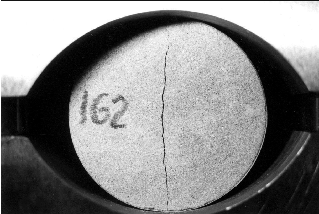
Figure 1-43: A BTS test after failure.
