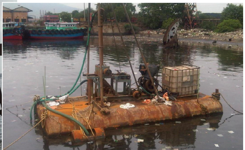
Figure 4-1 and 4-2: Good quality soil investigation cannot be performed with this type of equipment
