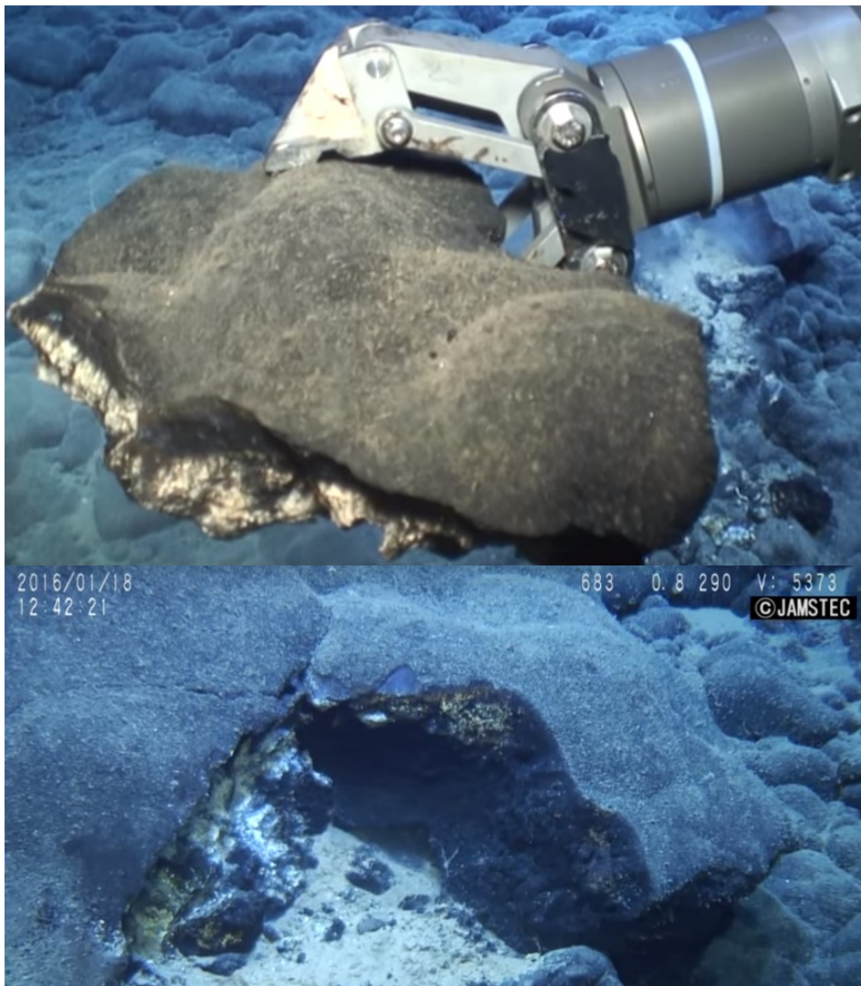
Figure 4: Piece of ferro-manganese crust (top) and cross-section of seafloor (bottom) from a seamount in the west Pacific (ca. 23°N, 153°E). Image Credit: Japan Agency for Marine-Earth Science and Technology 21 .
