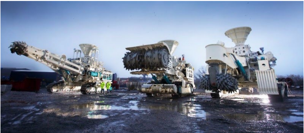
Figure 5: Mining vehicles designed to mine seafloor massive sulphides. Left to right: Collector machine, bulk cutter, auxiliary cutter. Image credit: Soil Machine Dynamics 24
